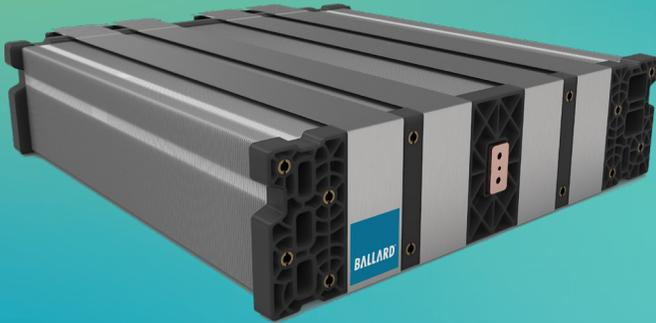
Ballard's FCgen®-LCS stack utilizes our proprietary heavy duty membrane electrode assembly (MEA) and low cost durable carbon plates to deliver performance and compelling total cost of ownership. This innovative design incorporates ports on both sides of our end plates for integration flexibility and provides stable electrical power scalable from 2.5kW to 93kW over a wide range of operating and environmental conditions.
