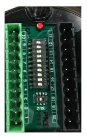
Fig. 18 DIP Switch Location
