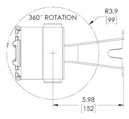
Fig. 13 FL500 and Mounting Bracket, Top View
