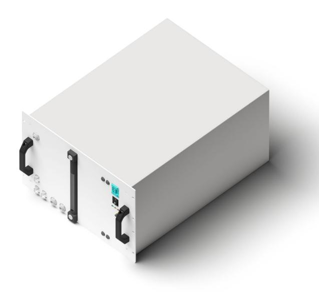
Enapter's Water Tank provides storage for 38 litres of clean water for the AEM electrolyser. The water tank is rack mountable into a standard 19" cabinet. The tank contains a conductivity sensor and a pump system to supply up to 11 AEM electrolysers with clean water.
