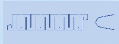
These standardized spring types are used in all U-shaped versions, such as the standard URI, URA, URS rod and piston seals and the URF shaft seals.
