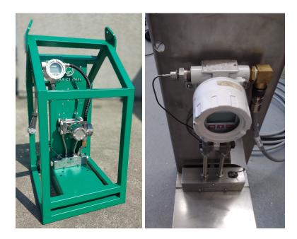
If supplied as a Rental meter, Hy-Cone comes equipped with 5300 or 10,000 psi rated differential pressure, static pressure and temperature elements and a choice of transport frame.
