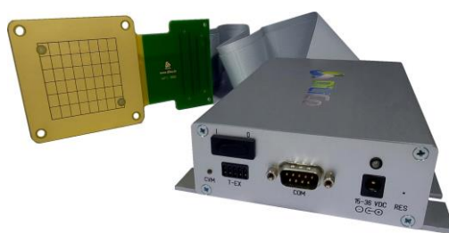
sensor layer with evaluation electronics
