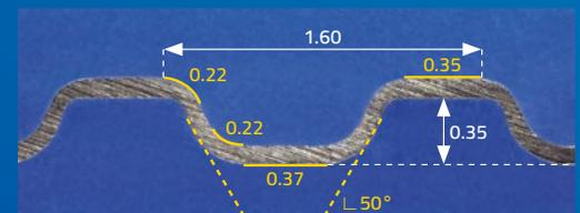
Foil thickness: 100 µm, Material: Alleima Sanergy® LT (316L)
