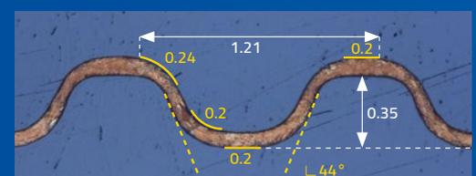
Foil thickness: 100 µm, Material: Titanium Grade 1
