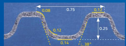
Foil thickness: 50 µm, Material: 304L
