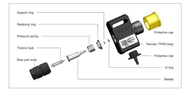
The Remote TPRD (Thermal Pressure Relief Device) is used to secure gas storage tanks in the event of a fire by ensuring rapid and spatially targeted degassing at elevated temperatures whilst preventing the tanks from bursting.
