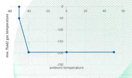
Derating of minimum medium (fluid / gas) temperature for low ambient temperatures.
