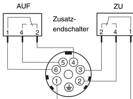
**12 V AC (Code B4) / 24 V AC (Code C4)****Belegung der Klemmleisten**
