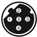
5-pin M12 built-in socket, D-coded
