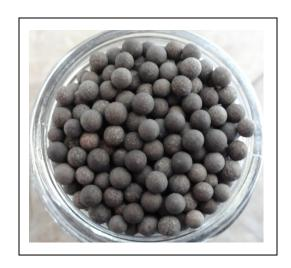
NOTE 1: Maximum recommended temperature for continuous operation is 500°C (932°F). Excursions above this temperature level should be minimized in order to obtain the maximum lifetime from this catalyst.
